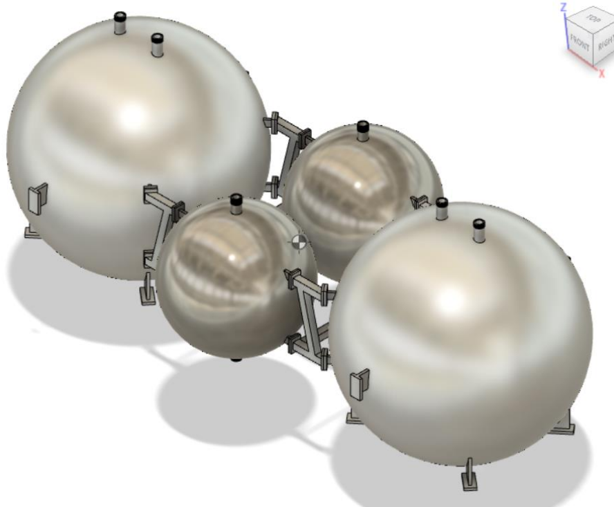
Figure 3. First Configuration. Methane tank (L); Oxygen Tank (R); Pressurizing Tanks (Front and Back)
