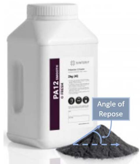
Figure 4.6: Angle of Repose (powder image from Sinterit website)
