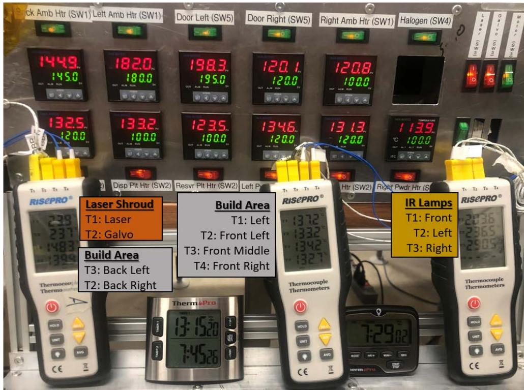
Figure 3.22: Tuned PID Setting for PA12 and PA12+CF and Internal Temperatures 13 hours and 15 Minutes into Print
