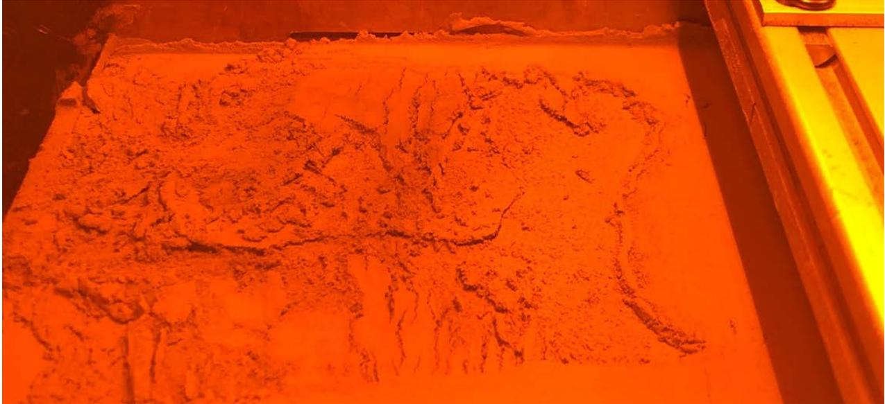
Figure 5.9: Example of powder degradation during extended vertical prints.
