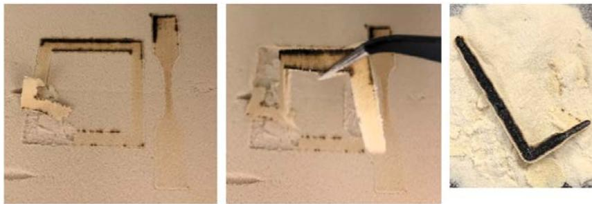
Figure 4.18: Laser power and wavelength unable to reach sintering window for PEEK. Laser energy is not sufficiently absorbed into the particles for affective heating and simply burns the top surface.
