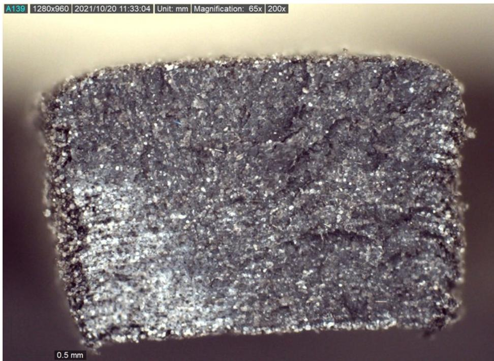
Figure 5.18: Fracture Surface of PA12 + 5% vol Carbon Fiber Horizontally Printed 3mmP Tensile Specimen
