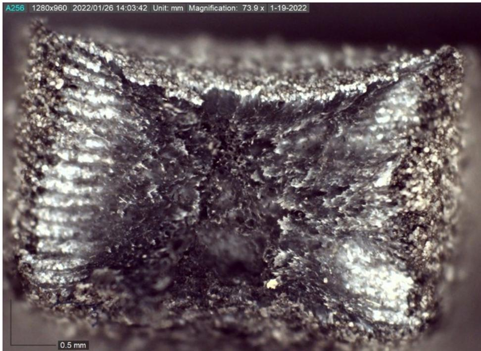
Figure 5.17: Fracture Surface of Neat PA12 (0% vol CF) Horizontally Printed 3mmP Tensile Specimen
