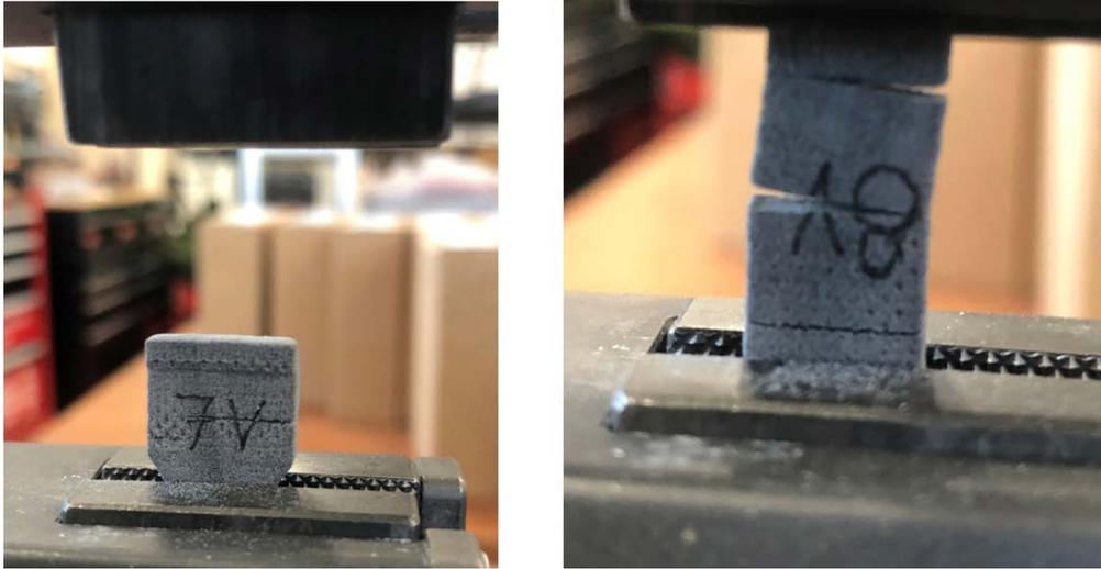
Figure 5.11: 10% CF vertically printed tensile specimen failure during grip insertion and initial pulling.
