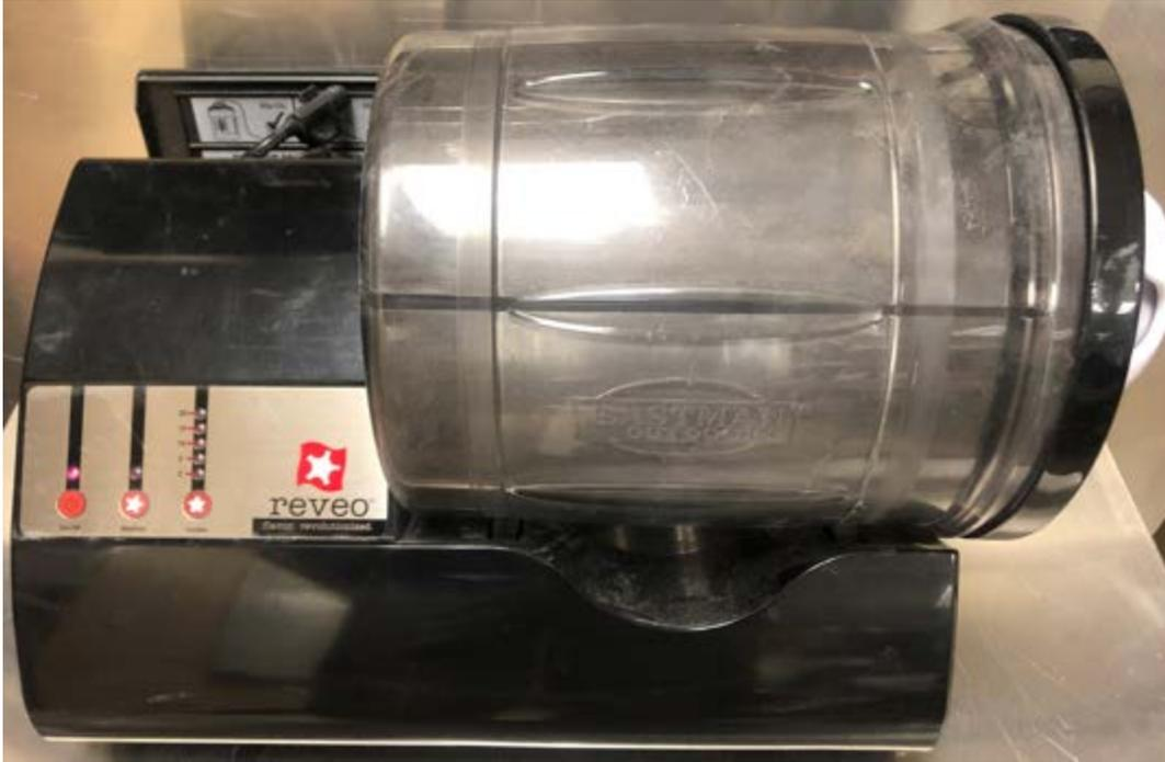
Figure 4.17: Mechanical tumbler used for all material blending.
