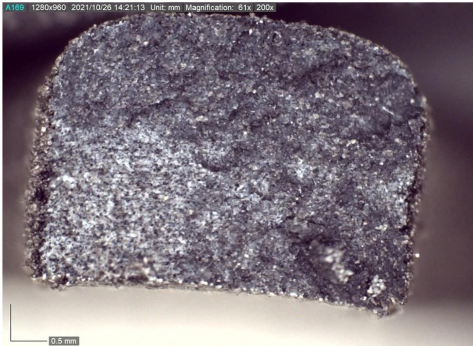
Figure 5.19: Fracture Surface of PA12 + 10% vol Carbon Fiber Horizontally Printed 3mmP Tensile Specimen
