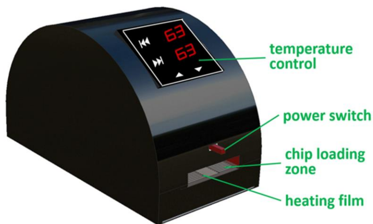
Figure 2.2: 3D schematic of the portable fully battery-powered heater. (Source: Adapted with permission from Duo et al. , 2019. Copyright @ 2018 The Elsevier. 38 )
