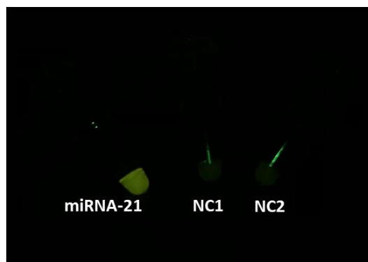
Figure 5.3: The off-chip detection of P-eRCA products from miRNA-21 and NCs under a portable blue light. Neither the NC tube showed notable fluorescence. miRNA-21: P-eRCA product from miRNA-21 sample ( 6 \times 10^4 copies); NC1: omission of padlock probe; NC2: omission of miRNA-21.
