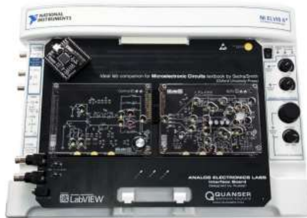
Figure 3 Analog Electronics Lab (AELabs) for NI Elvis [4] This system is a great option to prove basic concepts for analog circuits although it leaves a tiny degree of freedom to the user meaning that user cannot design their own prototype or circuit configuration to study.
