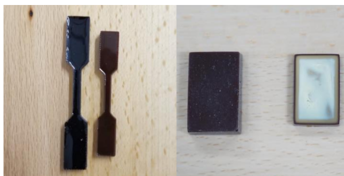
Figure 3.4.2.5.3: Changes in volume (A) and color (B) of PEG-vitrimer composite before (left) and after (right) exposure water and air drying.
