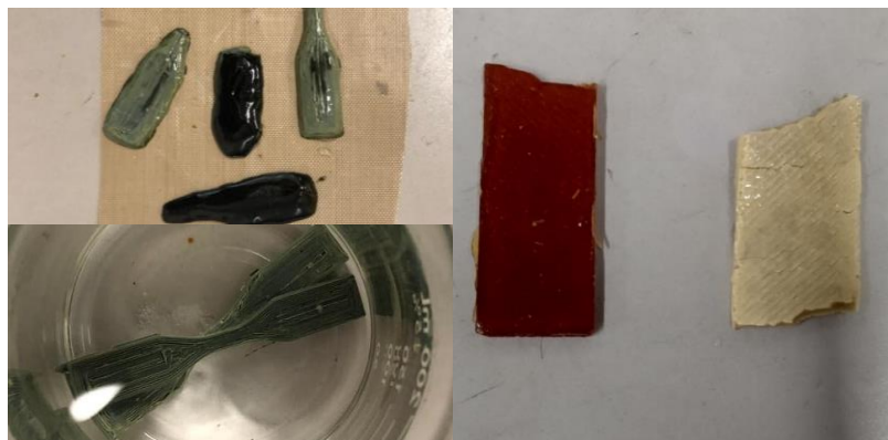
Figure 3.4.2.5.1: Discoloration of extruded (A, B) and casted (C) PEG-vitrimer composites.
