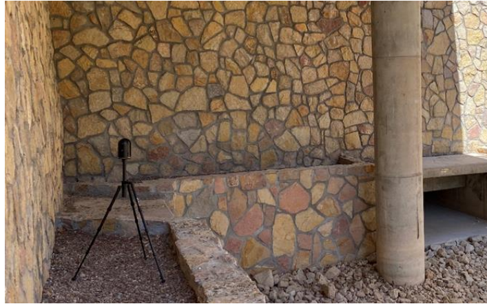
Figure 3. Photo. Set-up of Terrestrial LiDAR Scanner (BLK 360)
