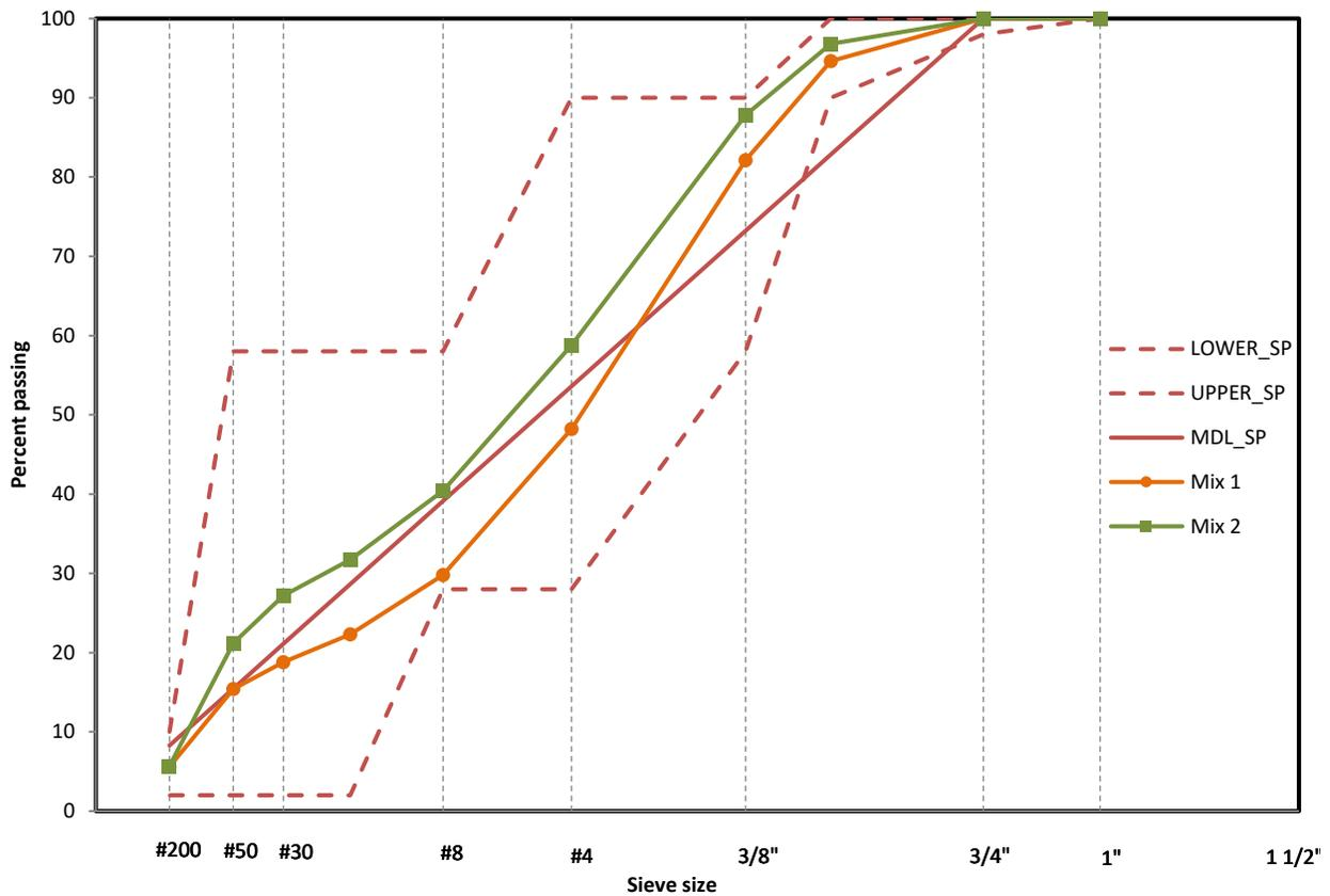
Figure 5-9 Particle size distribution of test section 5 mixtures
