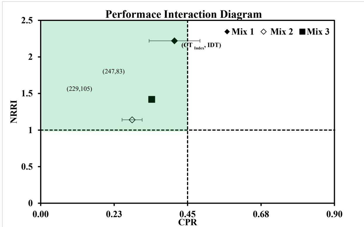
**Figure 5-6: Performance interaction diagram for test section 3 mixtures**
