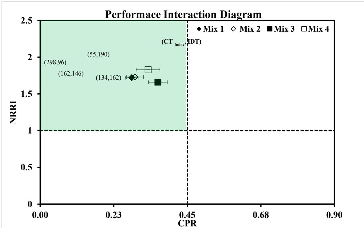
**Figure 5-8: Performance interaction diagram for test section 4 mixtures**
