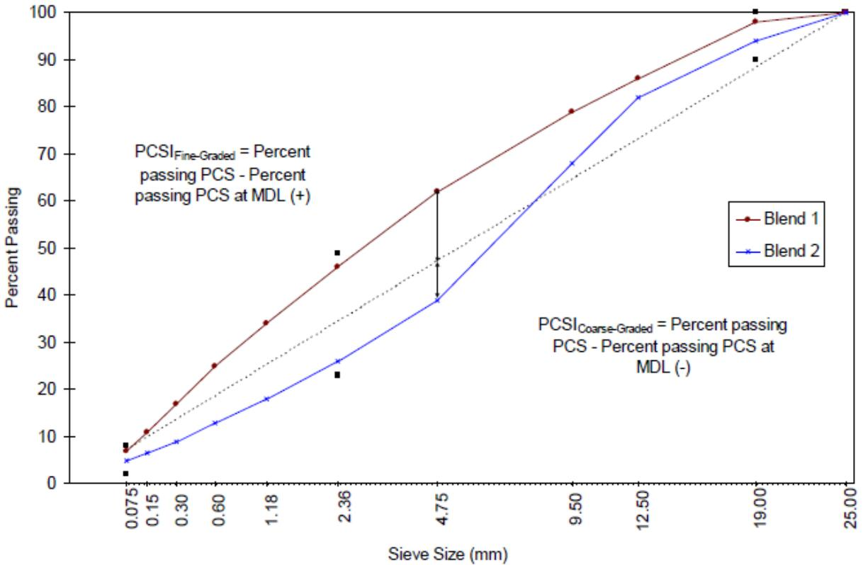
Figure 2-4: Illustration of PCSI for 19.0 mm NMAS gradations (Source: Leiva and West, 2021)
