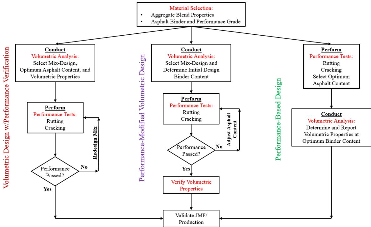
**Figure 2-5: Balanced mix design approaches (Source: West, R., 2018)**
