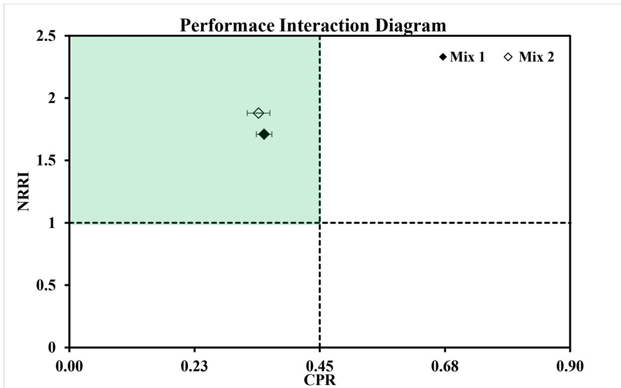
**Figure 5-10 Performance interaction diagram for test section 5 mixtures**
