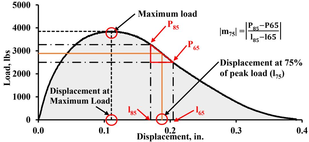
Figure 3-2 Performance tests and analysis methodologies
