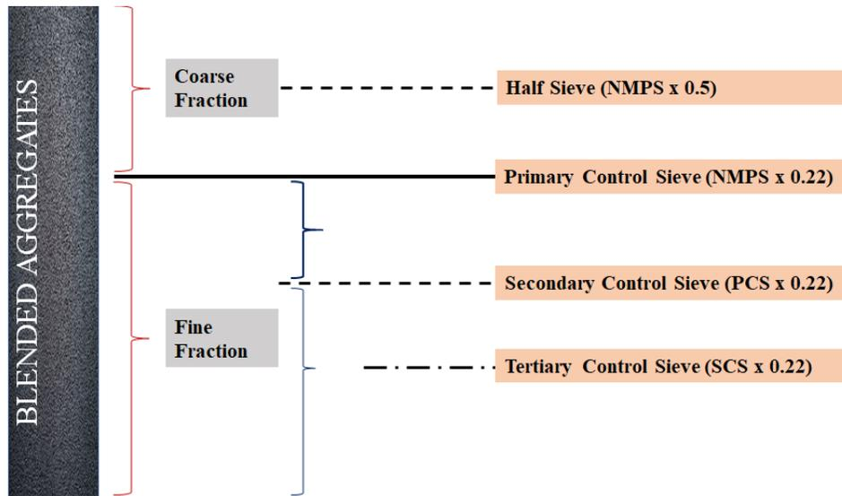
**Figure 2-3: Visual representation of aggregate gradation parameters**
