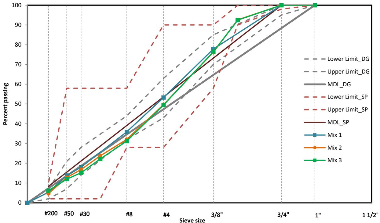
**Figure 5-3 Particle size distribution of test section 2 mixtures**
