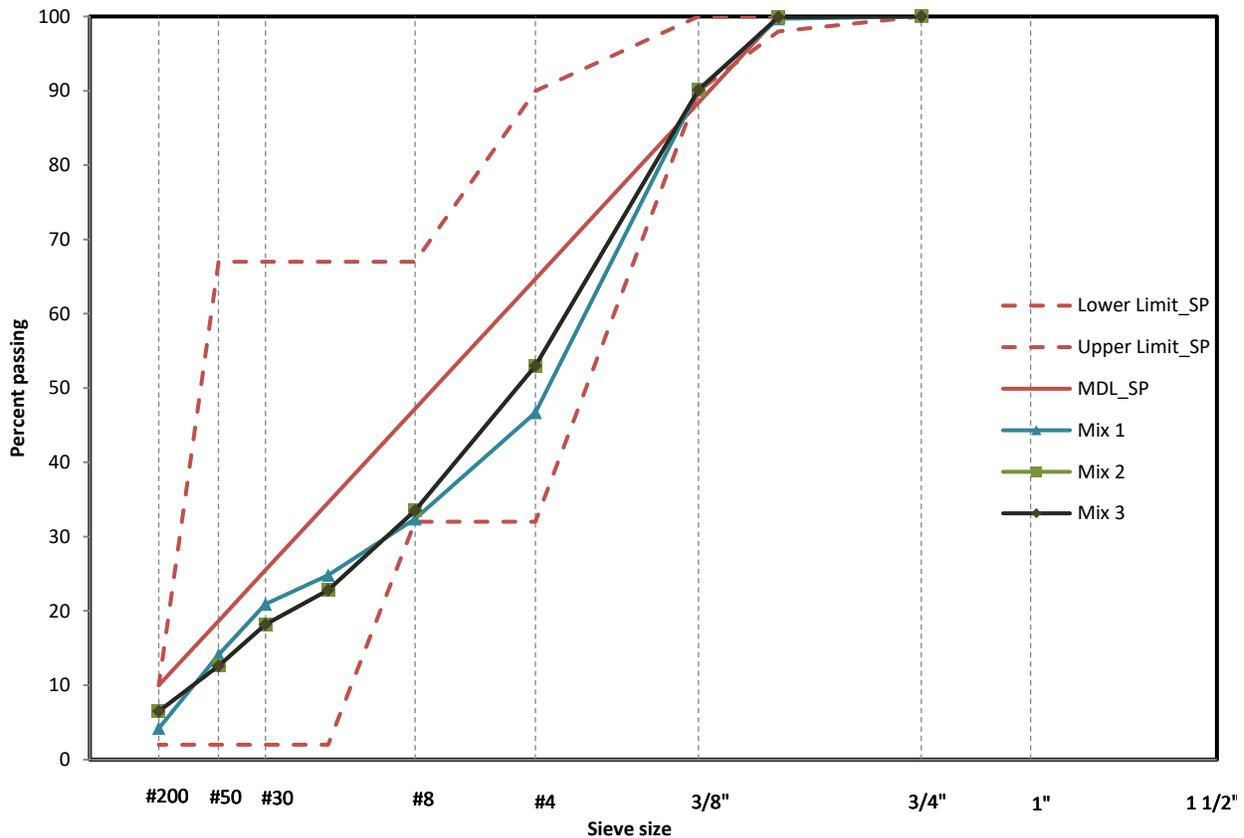
**Figure 5-5 Particle size distribution of test section 3 mixtures**
