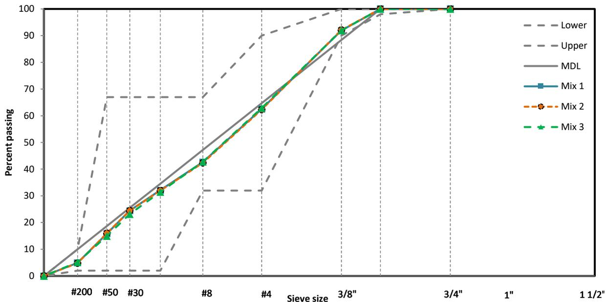
**Figure 5-1 Particle size distribution of test section 1 mixtures**
