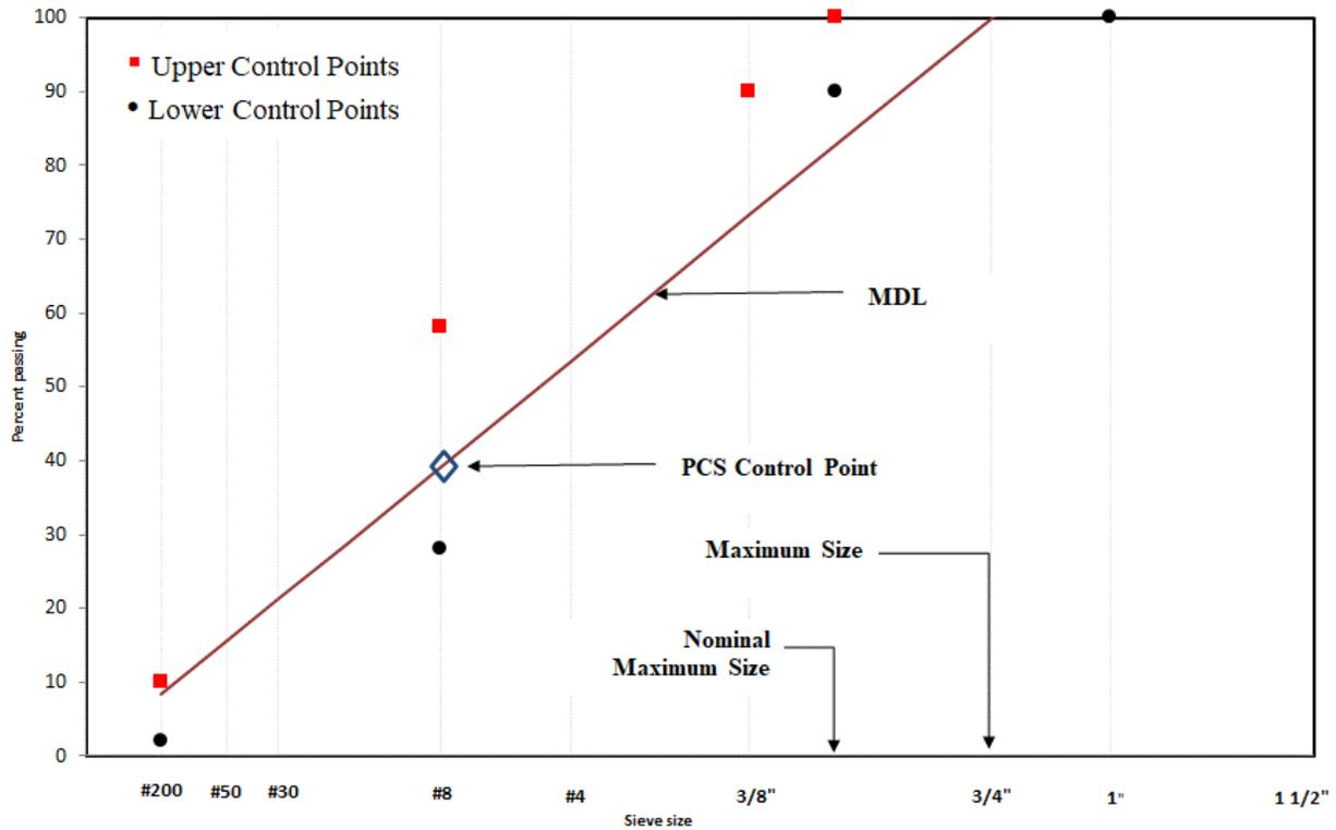
**Figure 2-2: Gradation control points and PCS point for 12.5-mm NMA**
