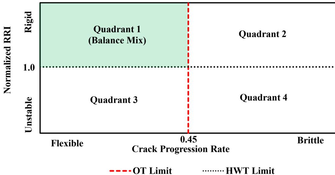
**Figure 2-6: Performance space diagram for balanced mix design**
