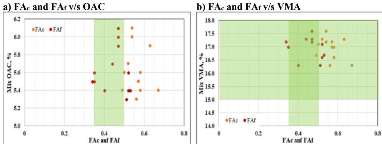
**Figure 6-5 Influence of  $FA_c$  and  $FA_f$  on the mix volumetric properties**
