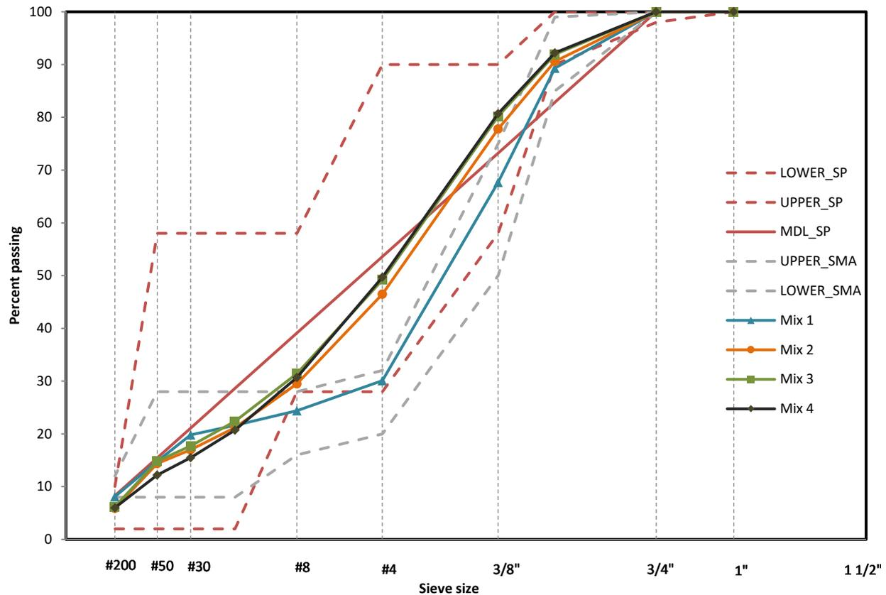
Figure 5.7 Particle size distribution of test section 4 mixtures
