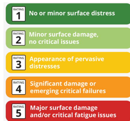
Figure 2.14 RoadBotic's Ratings for road conditions (RoadBotics, 2020)
