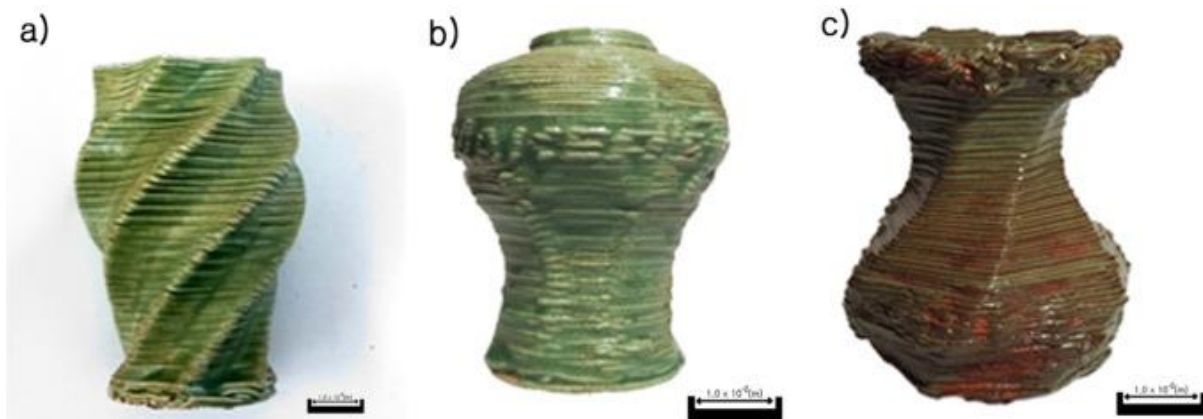
Figure 2.2 3D Printed enameled potteries of Ceramics using STE 3D Printing Technology. [77]
