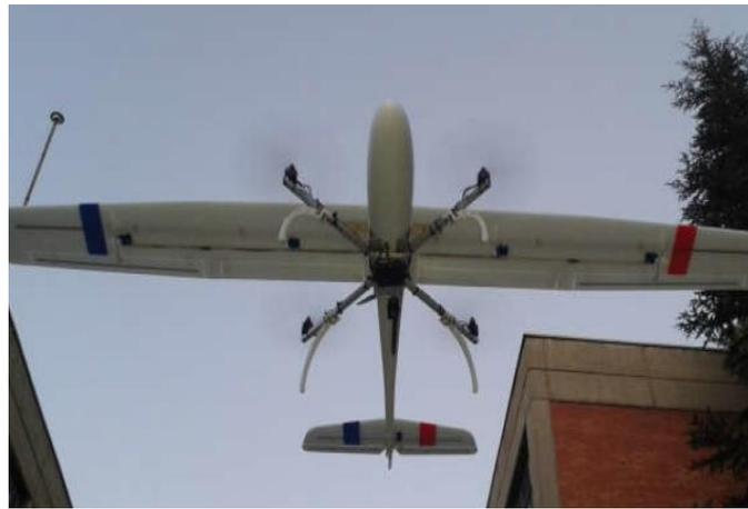
Figure 1.7: VTOL-FW UAV X-Way Fixed Bar (Cakici & Leblebicioglu, 2016)
