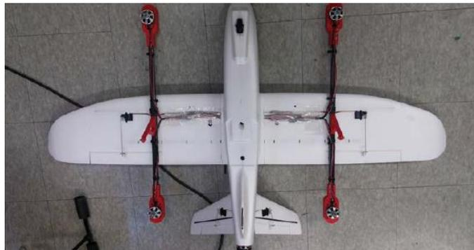
Figure 1.8: VTOL-FW UAV 11-Way Fixed Bar (Yu & Kwon, 2017)
