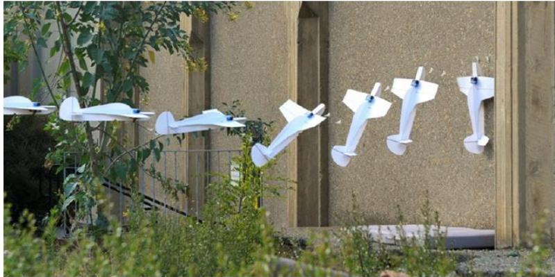
Figure 3.9: Perching Tail-Sitter UAV (Marchini, 2013)
