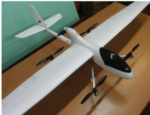
Figure 1.6: Vertical Take-Off and Landing Fixed Wing UAV (Cakici & Leblebicioglu, Analysis of a UAV that can Hover and Fly Level, 2016)
