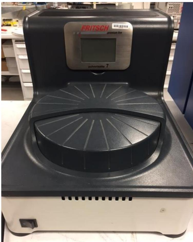
**Figure 3.4:** Planetary ball mill (Fritsch Pulverisette 7 Premium Line).
