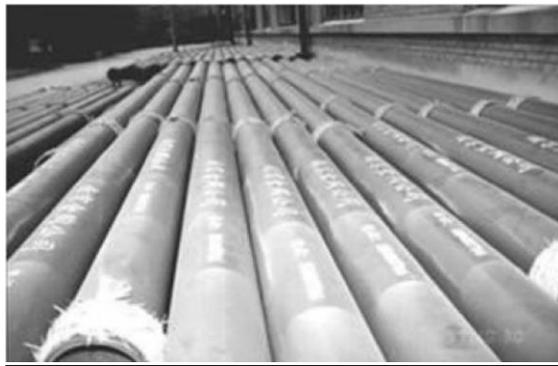
**Figure 2.4:** Large-scale ceramic-lined steel pipes produced using SHS [17].
