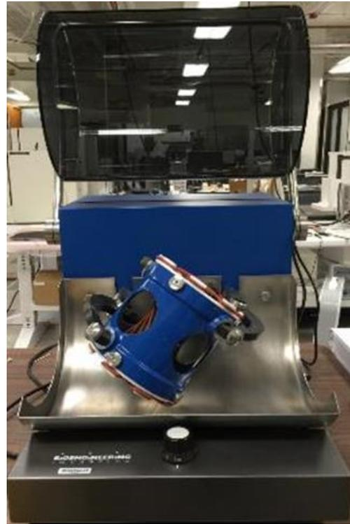
**Figure 3.1:** Mixer (Inversina 2L, Bioengineering) with (a) closed and (b) open protective shield.
