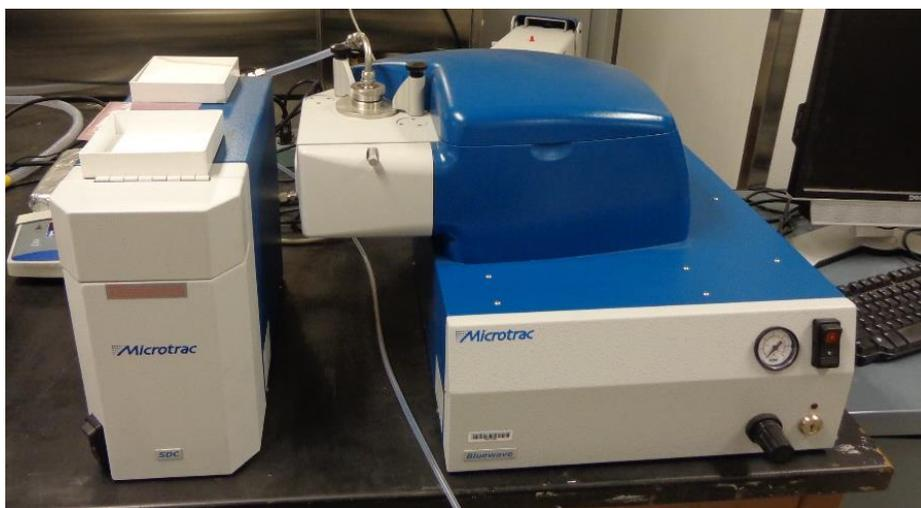
**Figure 3.7:** Particle size analyzer (Microtrac Bluewave).
