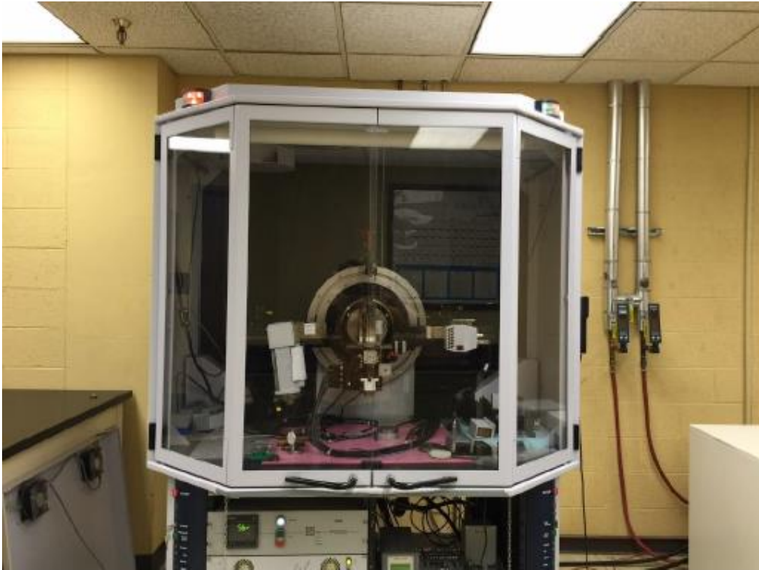
Figure 3.5: X-ray diffractometer (Bruker D8 Discover XRD).
