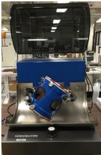
Figure 3.1: Mixer (Inversina 2L, Bioengineering).
