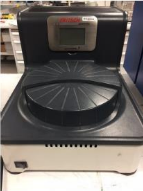
Figure 3.2: Milling equipment (a) planetary mill (Fritsch Pulverisette 7 Premium Line) and (b) grinding bowl with purging valves.
