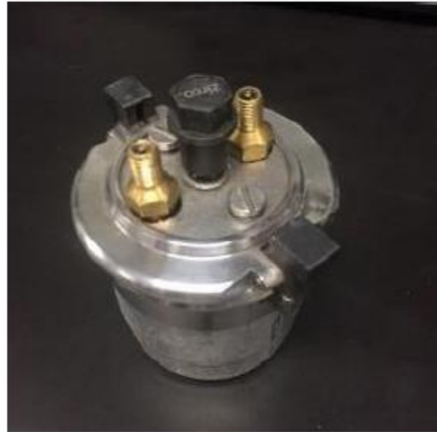
Figure 3.2: Milling equipment (a) planetary mill (Fritsch Pulverisette 7 Premium Line) and (b) grinding bowl with purging valves.
