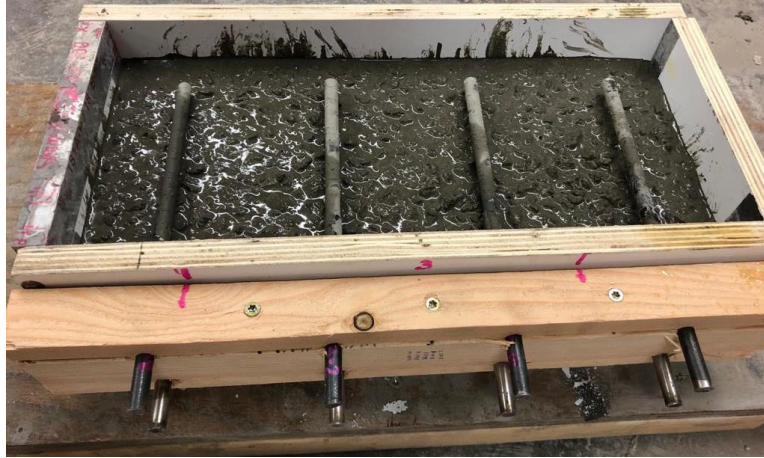
Figure 3.1 Concrete Specimen Preparation
