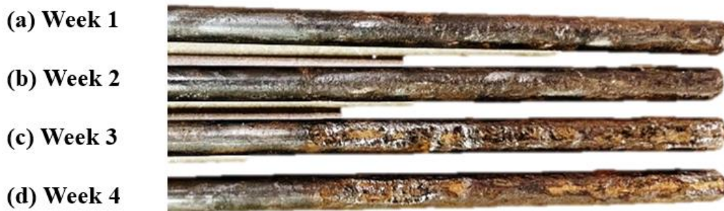
Figure 4.9 Progression of Corrosion of Carbon Steel Rebars with Duration of Submergence
