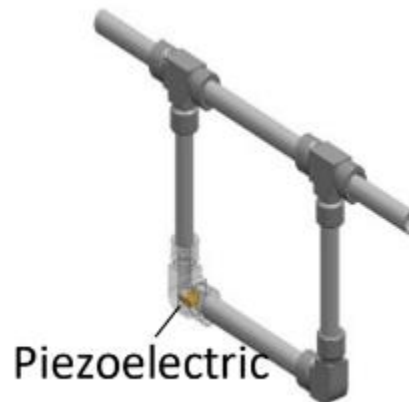
Figure 1.3.2: Bypass valve representation for HYPER facility
