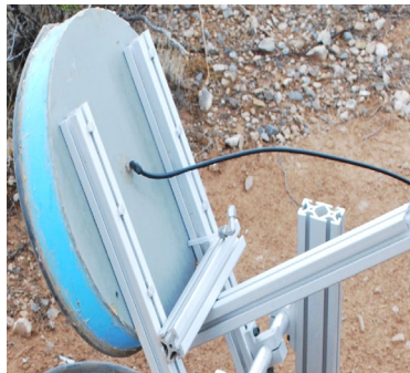
Figure 2.4 Lid assembly illustrating the connection of T-slot extrusions to the PVC aerobic
