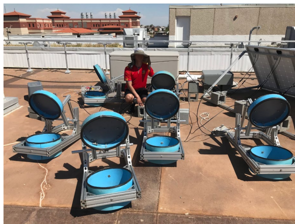
Figure 2.9 Connecting and testing the six automated flux chambers at the Green Roof of the Biology Building at UTEP.
