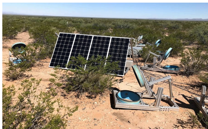
Figure 2.7 Assembly of all six automated flux chambers at The Jornada LTER site
