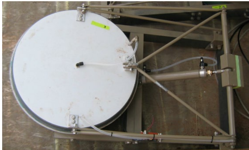
Figure 2.1 The original design of Ed Grote's automated flux chamber.
