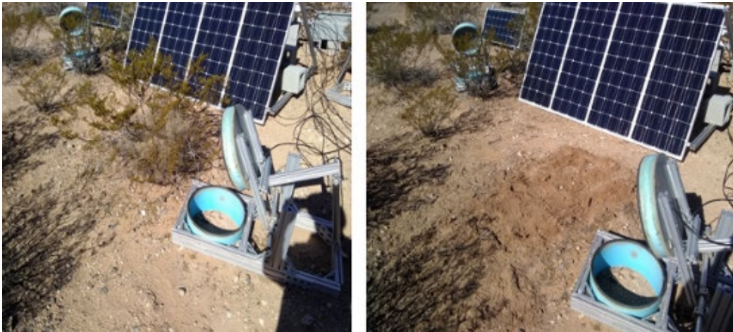
Figure 2.15 Automated flux chamber 2 before and after removal of creosote bush
