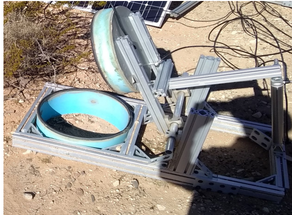
Figure 2.6 Attachment of the air cylinder to the lid and base of the automated flux chamber
