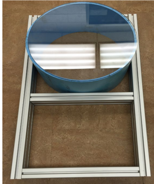
Figure 2.5 Attaching PVC Pipe to T-slot extrusions to build the base of the chambers
