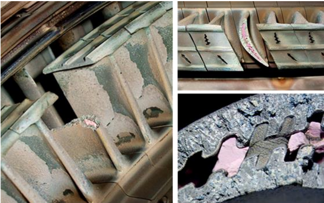
Figure 1.2 : Industrial gas turbine creep failure (Berkeley Research Company, Berkeley, California) [3]
