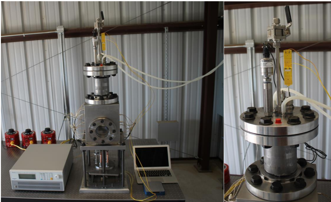
Figure 5.7: High Pressure High Heat Flux Pool Boiling Test Facility Assembly.
