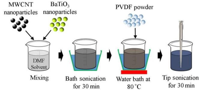
**Figure 4.1.** Solvent casting method of forming CNTs/BTO/PVDF nanocomposites.
