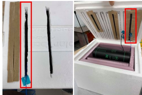
Figure 15: Exterior surface of the sample is only partially exposed while the opposing surface is completely exposed to the interior environment
