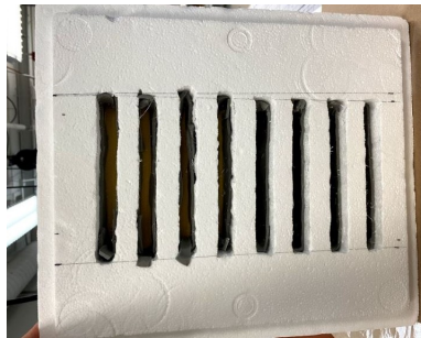
Figure 17: Configuration 3 samples are completely exposed to interior environment
