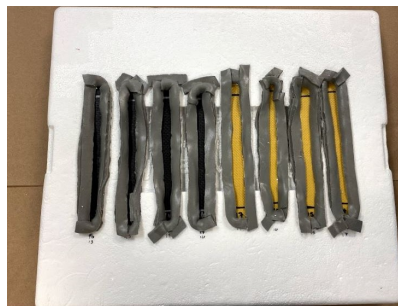
Figure 18: Configuration 3 samples are completely exposed to exterior environment
