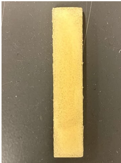
Figure 41: Method 1 resin sample with visible air bubbles on its surface
