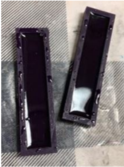
Figure 40: 3D printed cast resin molds for sample manufacturing
