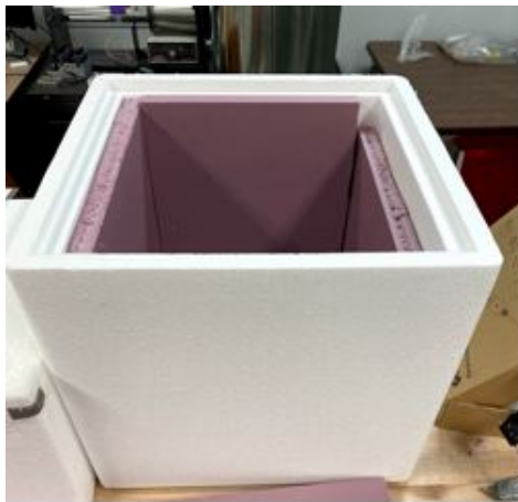
Figure 9: Chamber interior lined with a layer of polyurethane sheet foam insulation
