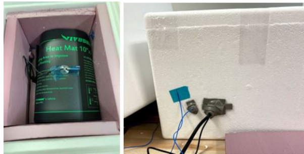
Figure 11: Heat source placed in insulated chamber interior and chamber wall view from cord and thermocouple incisions
