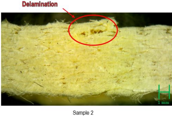
Figure 35: Microscope view of Kevlar fiber room temperature failure mechanism
