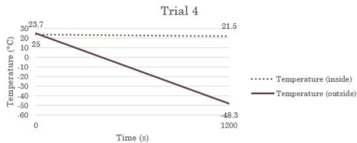
Figure 12: Environmental chamber interior is insulated and a heat source is integrated in trial 4 to test ability to maintain room temperature conditions
