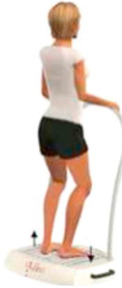
Fig. 2. Schematics of (a) the whole-body vibration timeline and protocol breakdown and (b) participant set-up on the side-alternation vibration platform. Vibrations were delivered intermittently at a frequency of 20 Hz and a vibration amplitude of 1.3mm.
