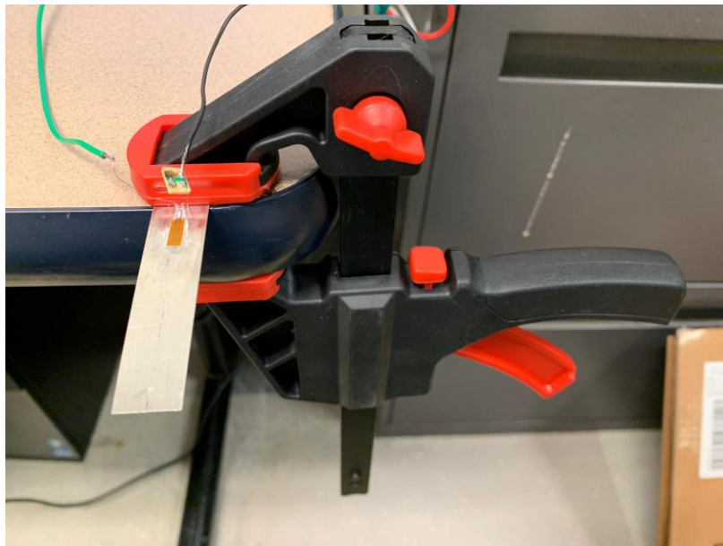
Figure 19 Strain gauge attached to a cantilever beam
