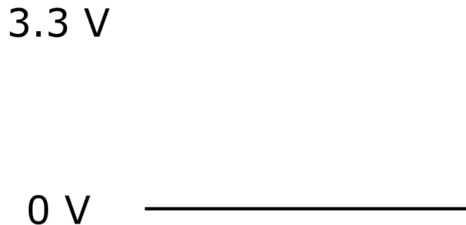
Figure 3.2: Example of a logic 0.
