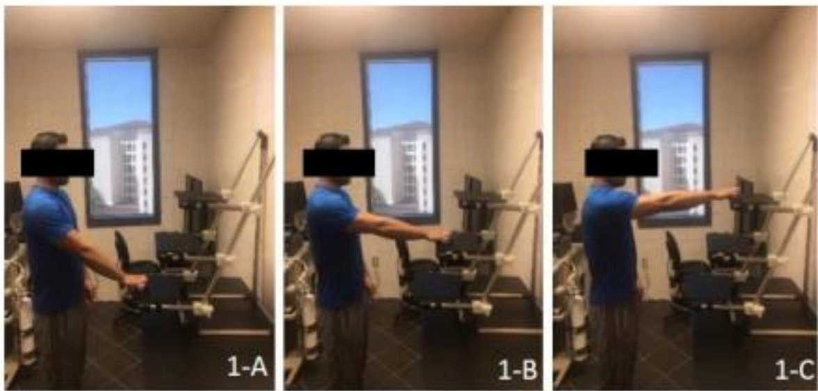
Figure 4. Location of the three different levels: shoulder at about 45°, 68°, and 90° angle. Participants moved a 0.5 lb. ball up and down until 1,800 cycles were completed.
