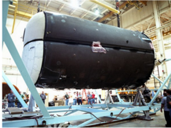
Figure 2: X - 33 Douglas, McCarville. “X-33 composite liquid hydrogen (LH2) tank failure” NASA Technical Reports Server, 28 Aug. 2017, https://ntrs.nasa.gov/search.jsp?R=20170012407
