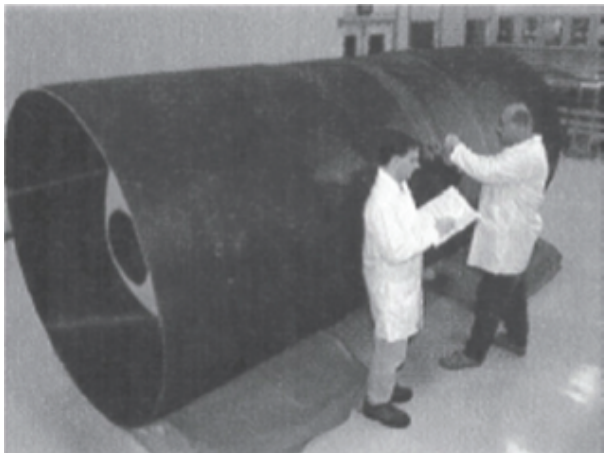
Figure 3: Space Launch Initiative Composite Cryotank Zheng, Hongfei. “DC-XA composite LH2 cryotank.” Intech Open, 14 March 2018, https://www.intechopen.com/books/solidification/the-application-of-carbon-fiber-composites-in-cryotank
