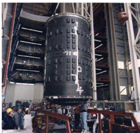
Figure 1: DC - XA Zheng, Hongfei. “DC-XA composite LH2 cryotank.” Intech Open, 14 March 2018, https://www.intechopen.com/books/solidification/the-application-of-carbon-fiber-composites-in-cryotank
