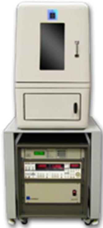
Figure 4.10: Hysitron 750 Nano-indentation System
