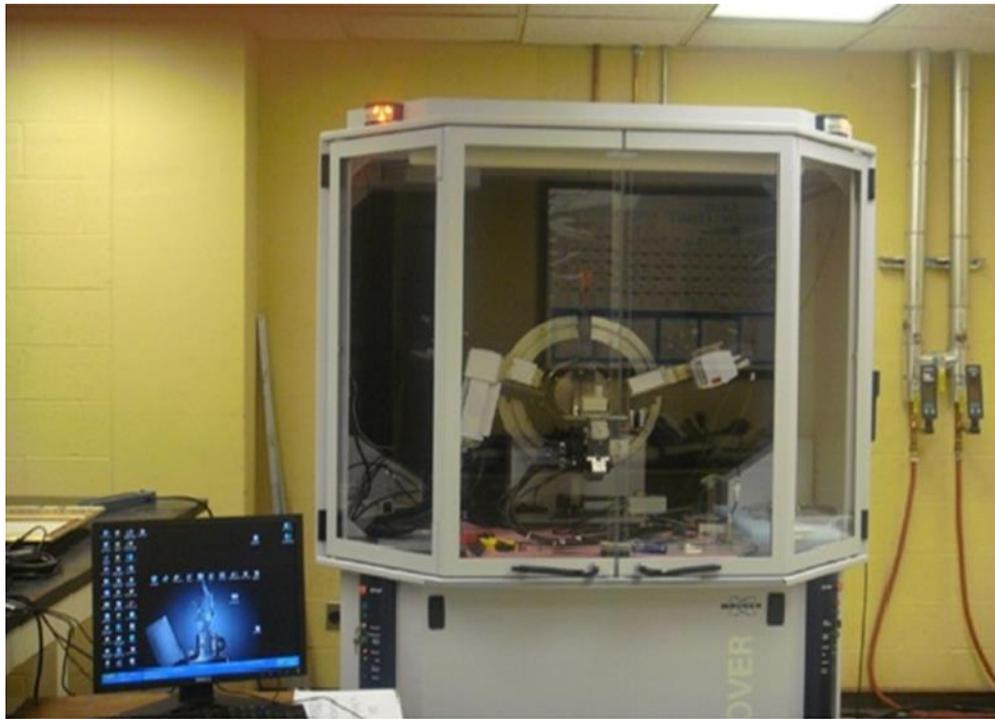
Figure 4.5: Bruker D8 Advance X-ray Diffractometer to characterize the  $\text{Ga}_2\text{O}_3$  and GMO films
