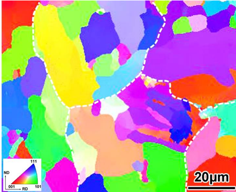
Figure 6. 2 Martensite orientation map of solution annealed parent steel.
