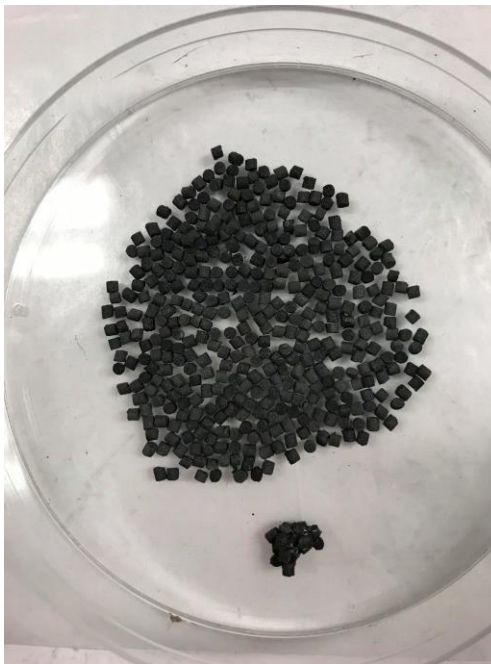
Figure 31: Silicon Carbide Catalyst Bed after Duty Cycle Testing with 0% of Pellets Fractured
