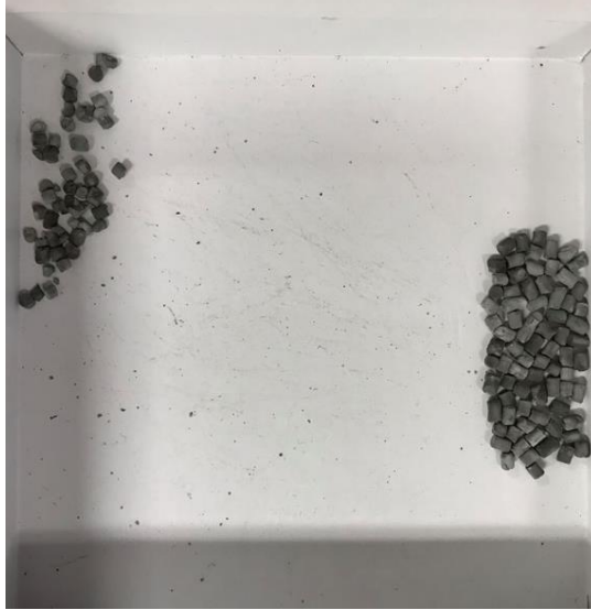
Figure 25: Aluminum Oxide Catalyst Bed after Duty Cycle Testing. 22% of Pellets Fractured
