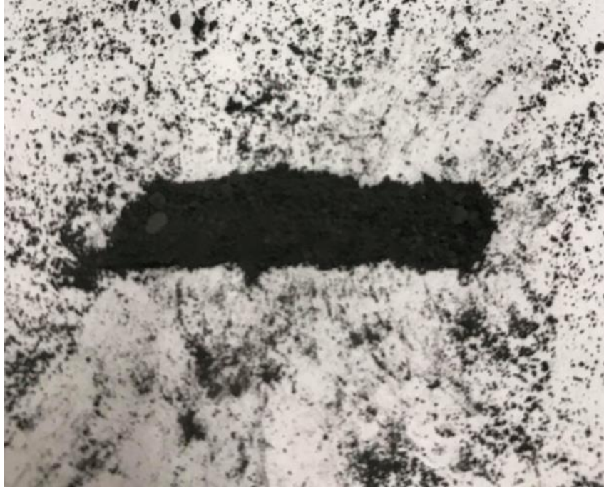
Figure 28: Tungstated Zirconia Catalyst Bed after Duty Cycle Testing. 100% of Pellets Fractured
