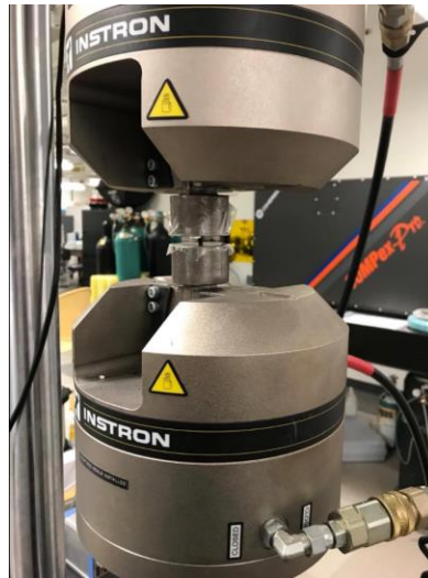
Figure 19: Compression Test Machine with Single Iridium Coated Alumina Pellet
