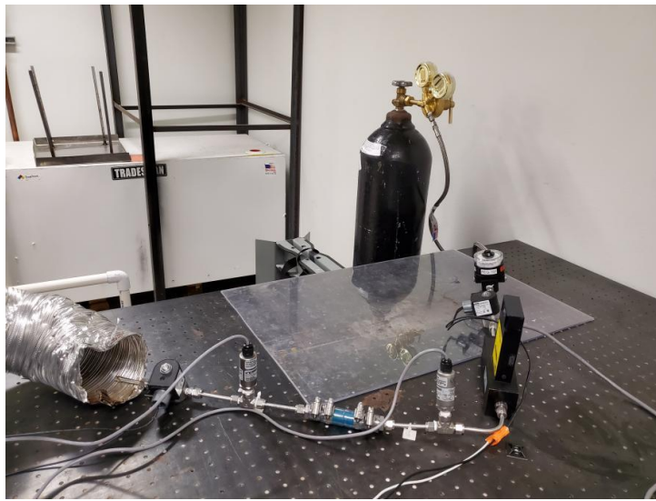
Figure 38: Lattice Pressure Drop Test Experimental Setup
