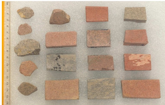
Figure 2.2 Polished blocks and specimens of pink (including red and purple hues) and gray varieties of Round Top Mountain rhyolite. Note sub-mm size of the mineral grains. Scale = 16 cm.
