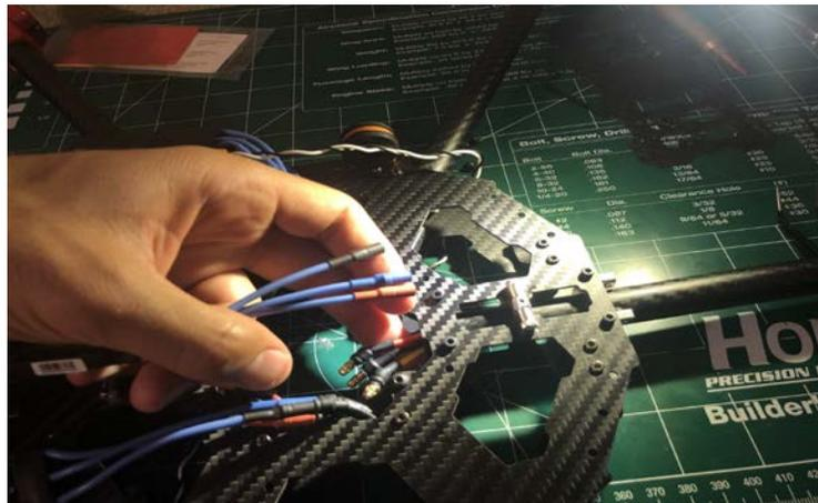
Step 7: install the electronic speed controller and circuit board to the carbon fiber frame with the included screws and zip ties, then test the connection with the multimeter
