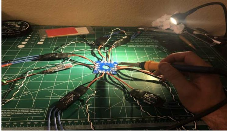
Step 6: connect the electronic speed controls to the motors: red to red, black to black, yellow to blue [clockwise]-red to black, black to red, and yellow to blue [counterclockwise]
