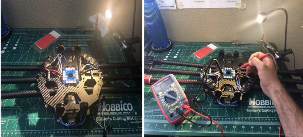
Step 8: mark each motor by number according to the motor rotation of the Hexacopter
