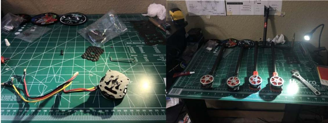
Step 4: connect the remaining four arms to the frame with the carbon fiber pipe buckle
