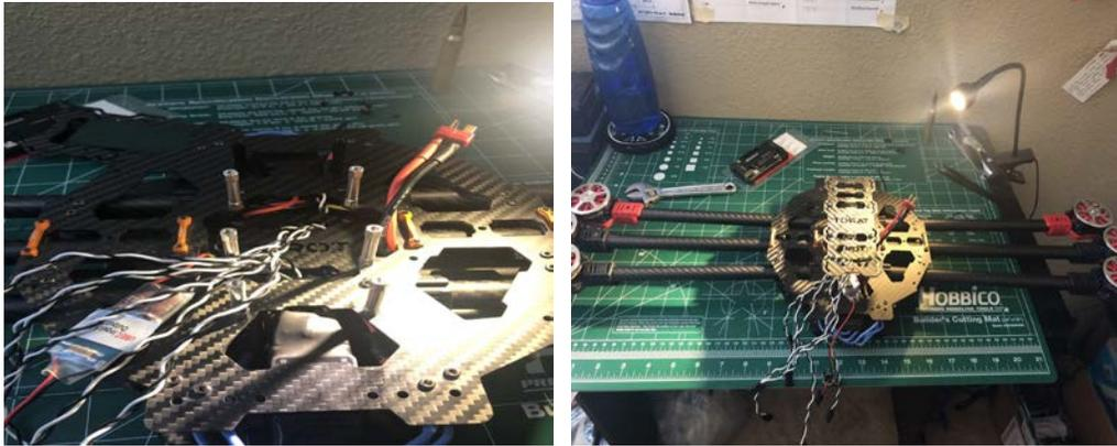
Step 10: connect the receiver to the flight controller along with the GPS system and power wire
