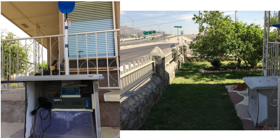
Figure 6 Air Quality Monitor Set-Up: Near-Road Home
