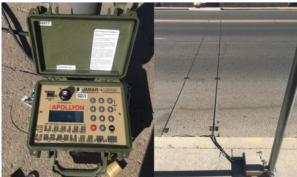
Figure 3 Tube Counters On-Site (Pershing Location)
