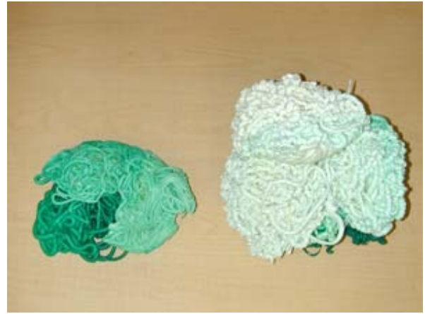
Figure 2: (b) Example of purge scrap
