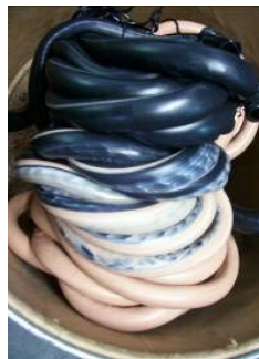
Figure 15: Example of color change scrap by purging of compound through extruder
