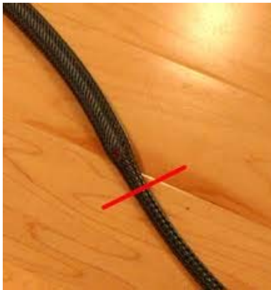
Figure 16: Example of Lump defect observed on the wire [20]
