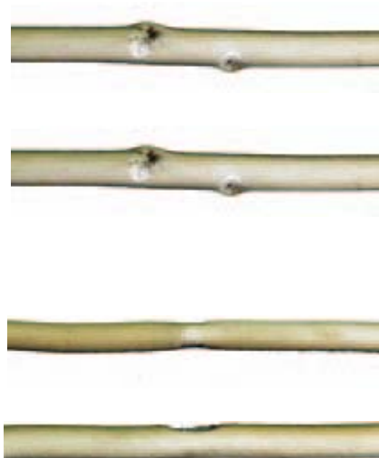
Figure 17: Example of spark out observed, mostly on small gauge wire
