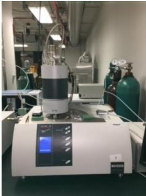
Figure 2.5: Netzsch DSC 404 F1 Pegasus Differential Scanning Calorimeter
