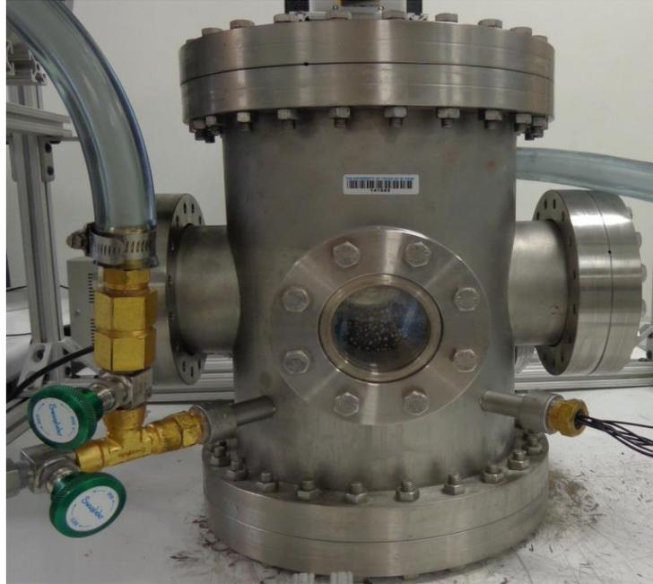
Figure 2.3: Laser Ignition Vacuum Chamber.
