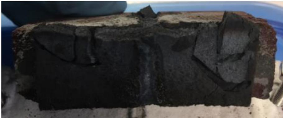
Figure 3.11: Joining of two 12.7mm tiles.
