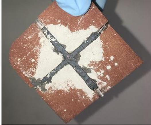
Figure 3.12: Joining of four 12.7mm tiles.
