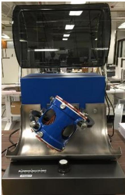
Figure 2.2: Inversina 2L 3-D Inversion Kinematics Mixer.
