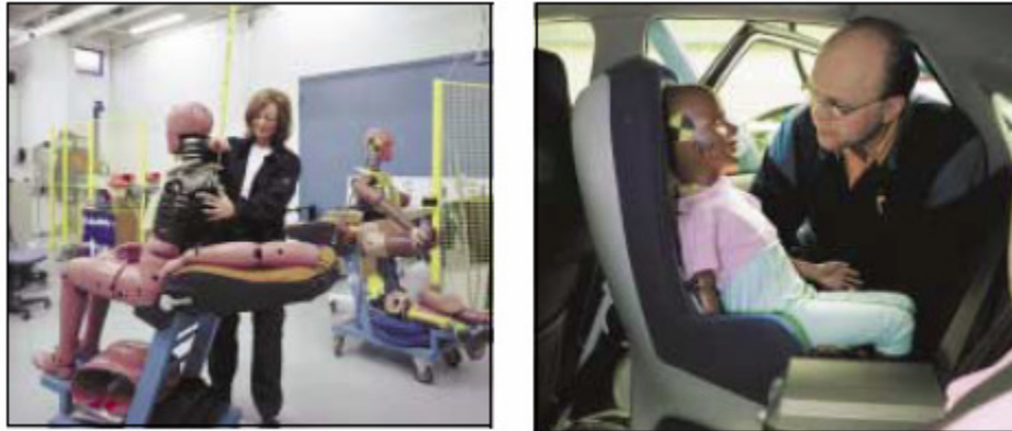
Fig 3.2: Preparation of dummies for crash test impact [37].
