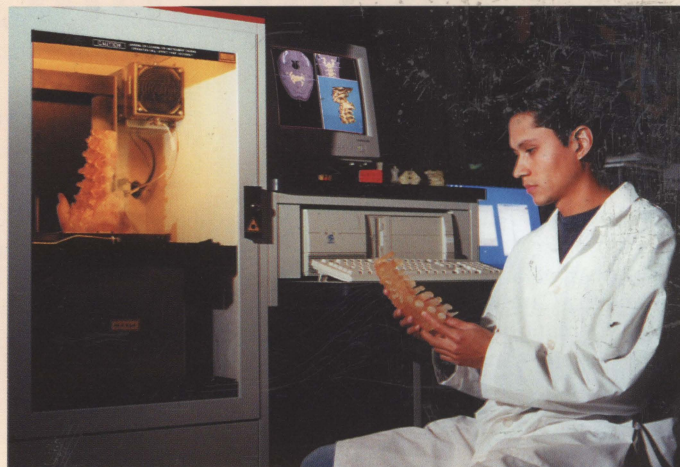
Ph.D. student Erasmo Lopez studies a model of a human spine created with the W.M. Keck Border Biomedical Manufacturing and Engineering Laboratory's rapid prototyping technology.
